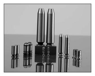
Confusion often arises when comparing headspace readings generated by gauges from different manufacturers--a rifle may accept both "GO" and "NO GO" gauges from one maker but only the "GO" from another. This would lead a reasonable person to ask, "why?" The answer lies in the dimensions and tolerances to which the gauges are made.
