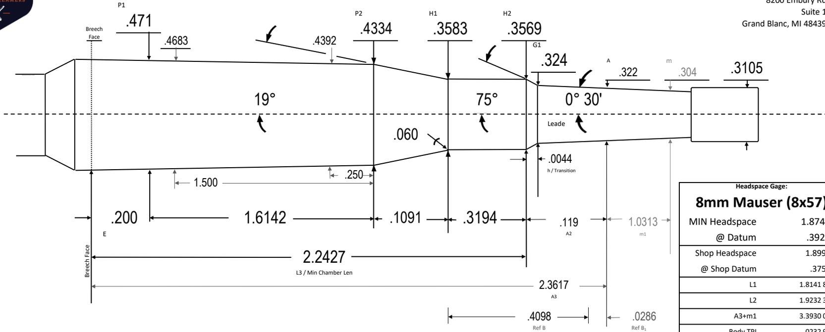
Chamber body & neck meets SAAMI 2015 spec vrfd 2/22/22rg, 24.01.14rg. D Manson modified lead to 0° 30'. SAAMI lead is 0° 25' 26"
