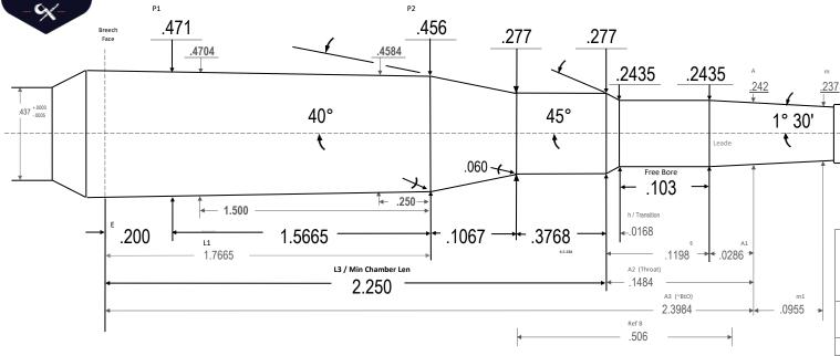
Ackley Improved version of 6mm Rem. Base diameter is slightly tightened. Free bore length remains the same as 6 Rem, but leade angle is changed to 1.5 degree (from 3 deg). Throat will be longer than needed for most 6mm/.243 bullets with the exception of some of the heavier (105+gr) hunting type bullets. Will shoot any traditionally loaded 6 Rem bullets as well as a standard 6 Rem would. Throat can be shortened to suit.
