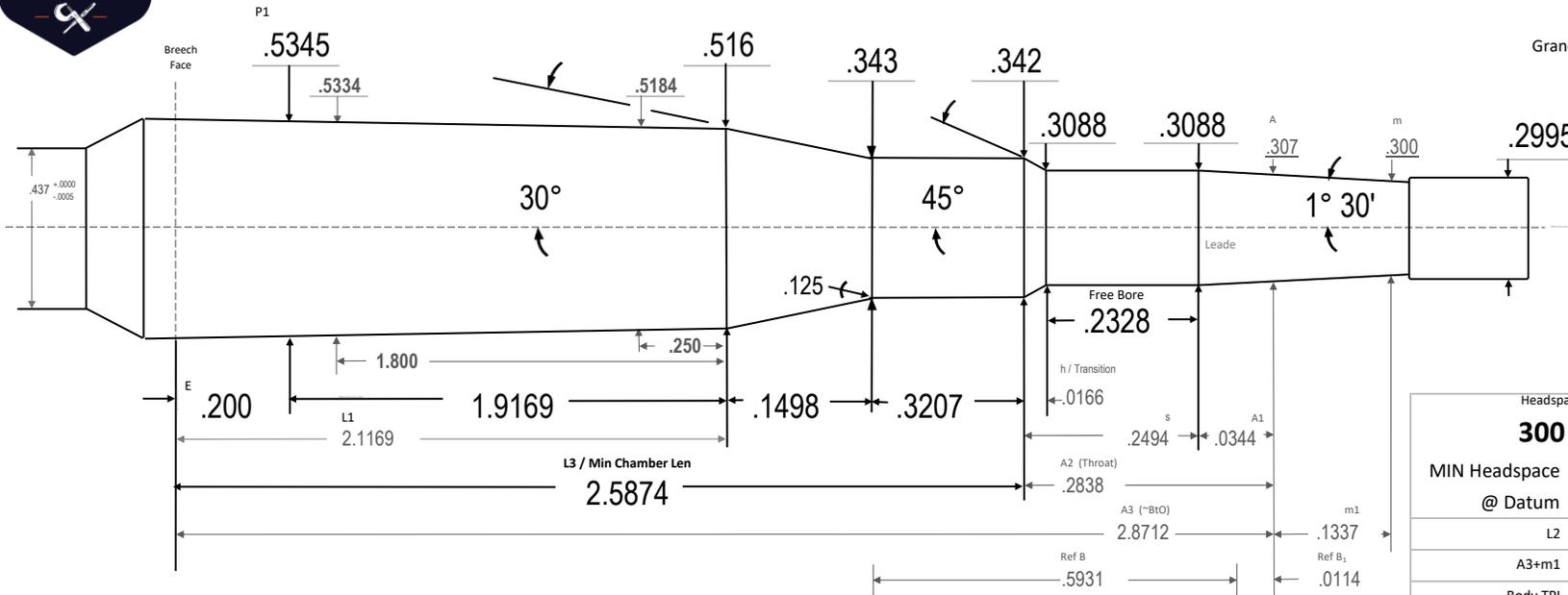
Chamber is minimum SAAMI spec with the exception of the larger base diameter, to address known extraction issues
